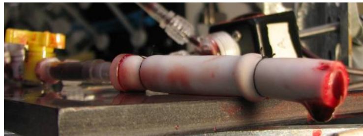
Figure 41: Dacron sleeve attached to non-pulsatile system
